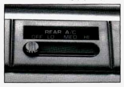
You may have rear air conditioning. The rear air conditioning switch is located above the radio at the top of the instrument panel. Slide the lever toward HI for cooler air in the rear area. Slide the lever to OFF to turn the system off.
